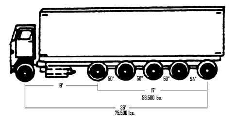
Steering Axle Weight 17.5" = 19,250 lbs 5 Axle Grouping Weights 58,500 lbs on state system with bridge length permit 48,000 lbs without permit 58,500 lbs on interstate system (I-29 & I-94) – no permit required
