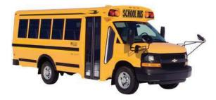
**Type B:** A Type "B" school bus is constructed utilizing a stripped chassis. The entrance door is behind the front wheels. This definition includes two classifications: **Type B-1**, with a GVWR of 10,000 pounds or less; and **Type B-2**, with a GVWR greater than 10,000 pounds.
