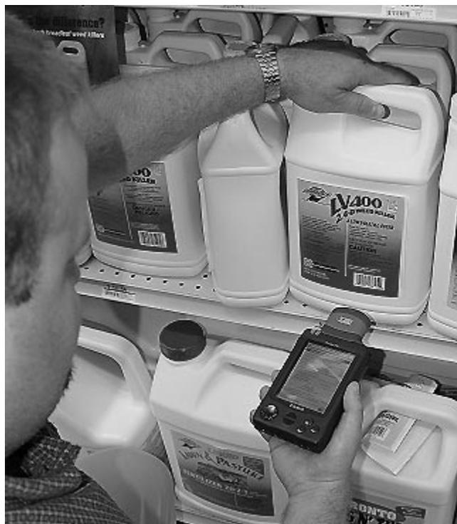
Handheld computers with built-in scanners enable NDDA inspectors to determine if pesticide products on the shelf have been properly registered.
