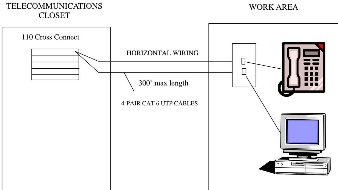
FIGURE 1.1 Typical Horizontal and Work Area Wiring
