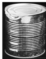
Dented at junction of side and end
