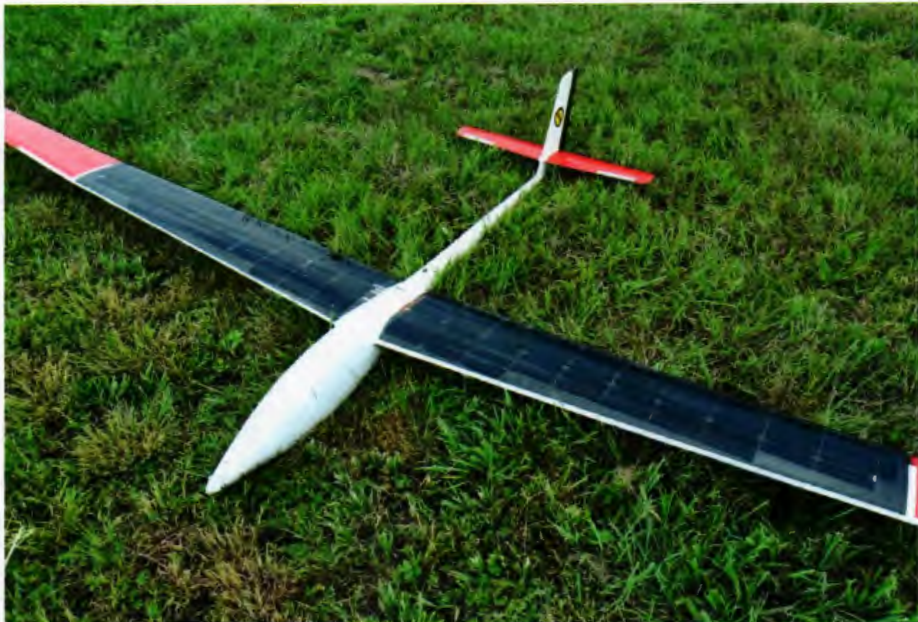
Figure 3: PV-SBXC aircraft with Si solar cells attached to the wings
