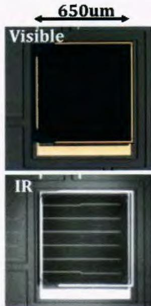
**Figure 1: Photograph of a stacked cell. Top picture (visible) shows the GaAs-based cells, the bottom figure (IR) shows the bottom, InP cells.**
