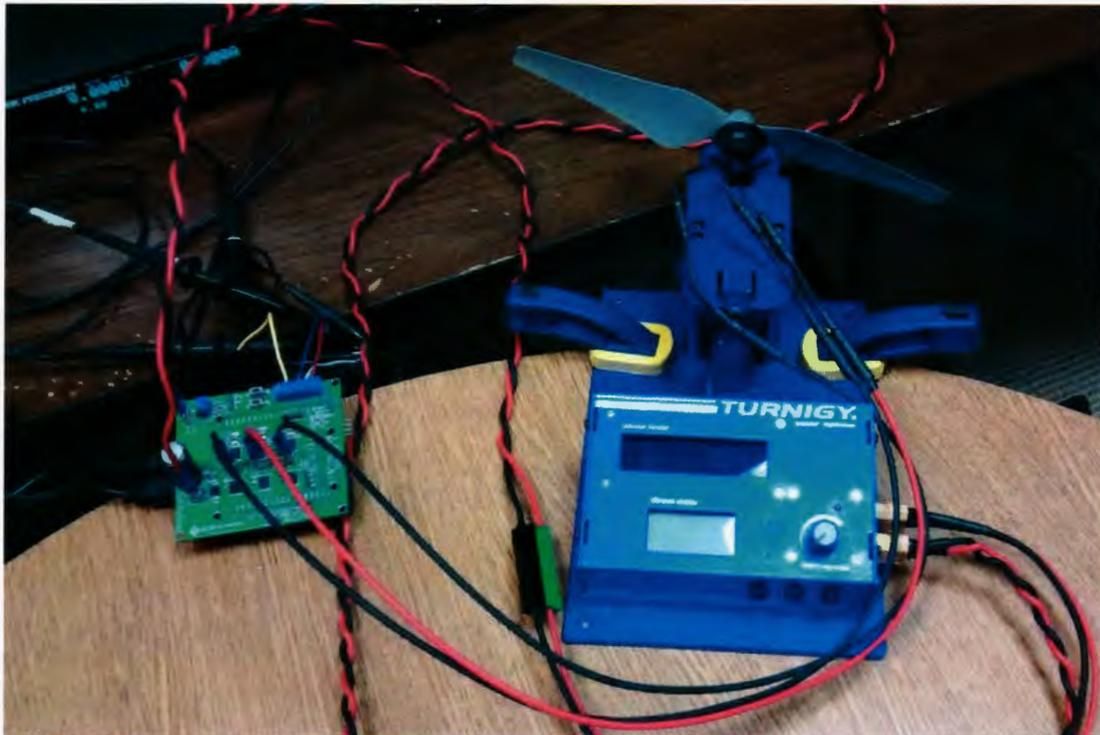
**Figure 8: ESC Prototype Board and Thrust Monitor**
