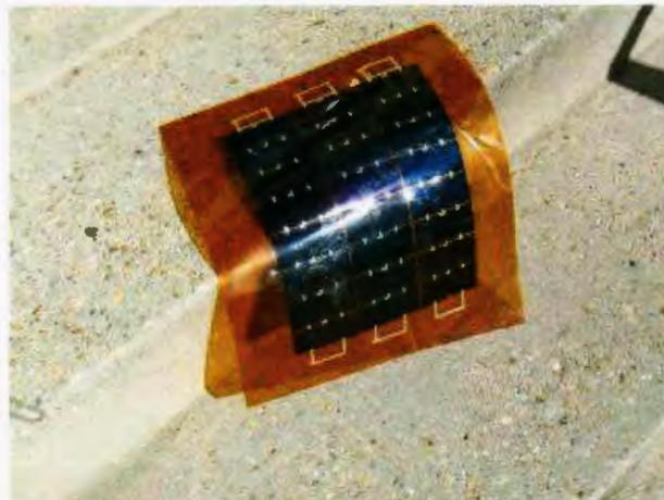
**Figure 2: Flexible solar array material being used to develop the UAV wing skin. This example uses multijunction, large area solar cells with flexible encapsulation.**
