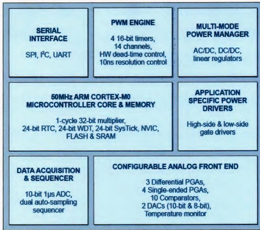
**Figure 7: Power Application Controller**
