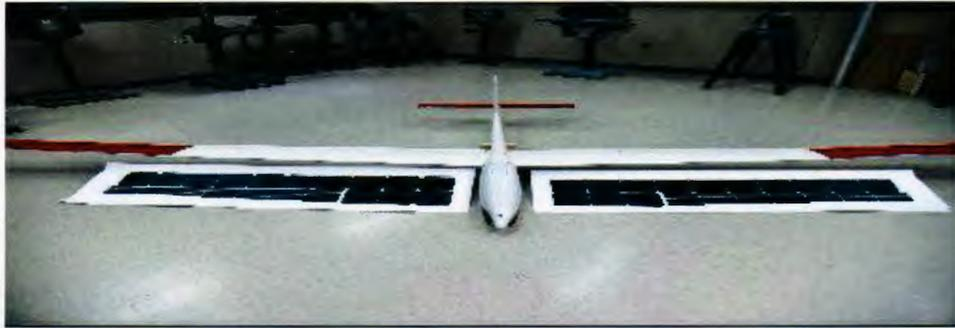
**Figure 3: A photo of the flexible Si arrays next to one of the UAVs. These arrays will be used as the wing skin for a new wing assembly.**
