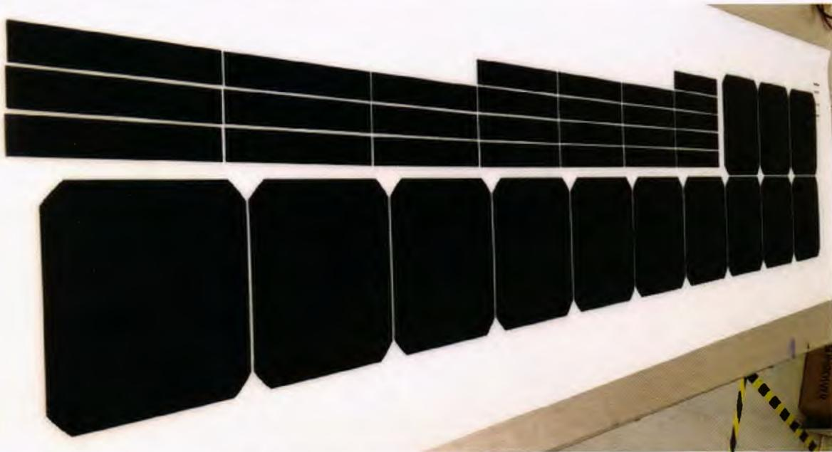
**Figure 3: Prototype cell layout (left wing half)**
