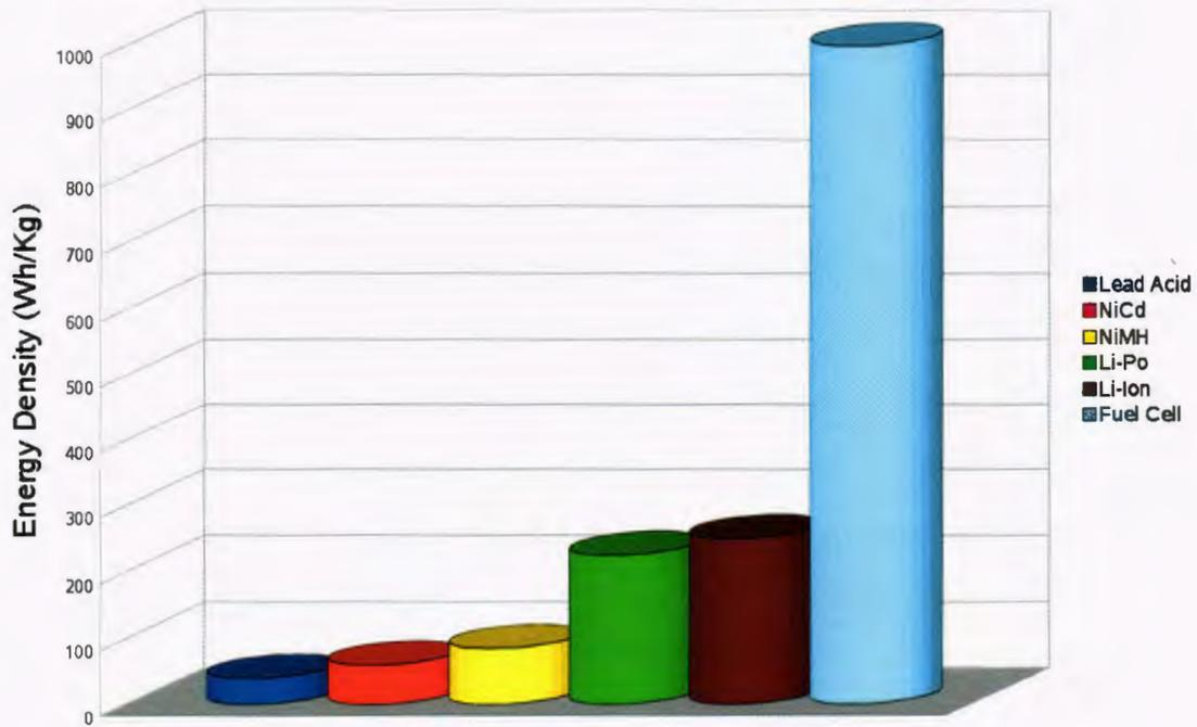
**Figure 6: Fuel cell energy density comparison**
