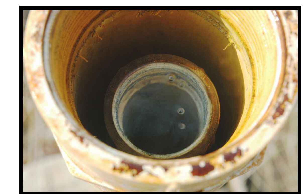
Figure 1. View of the TOC of observation well 162-83-15CCC showing methane gas bubbles rising through the water column at the top of the well. Diameter of PVC observation well containing gas bubbles is 2-in.
