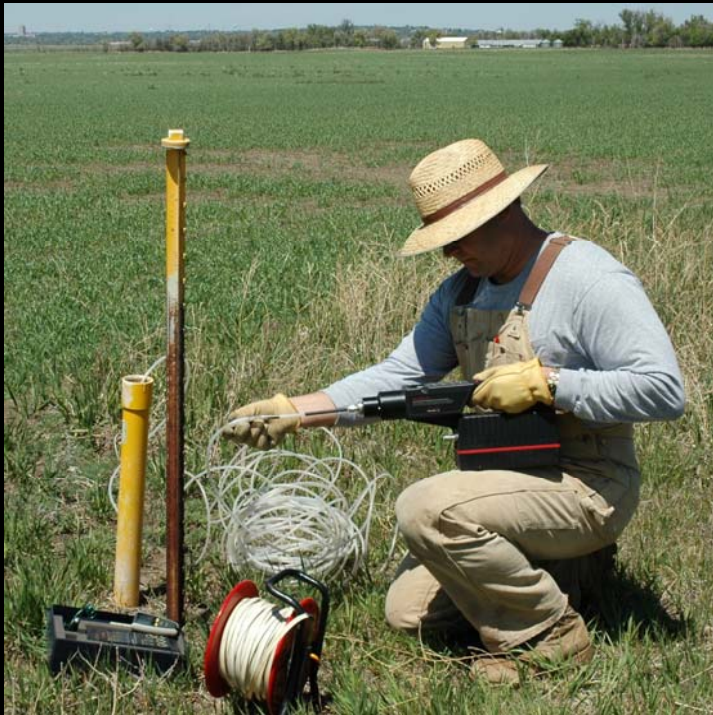
Field screening for shallow gas with a portable flame-ionization detector (FID) equipped with a an extended sample probe in Burleigh County N.D. in 2008.
