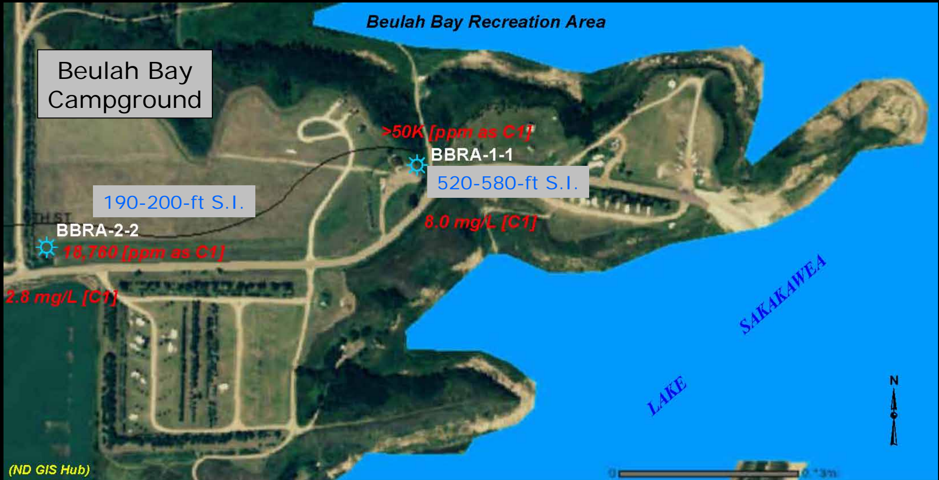
Locations of water supply wells at the Beulah Bay Campground where recent shallow CBM occurrences were reported.
