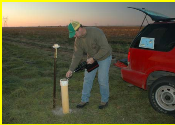
Field screening for shallow gas with a portable flame-ionization detector (FID) in Emmons County N.D. in 2006.
