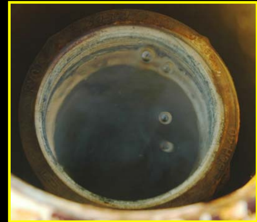
Methane bubbles in a shallow ground-water observation well in Bottineau County
